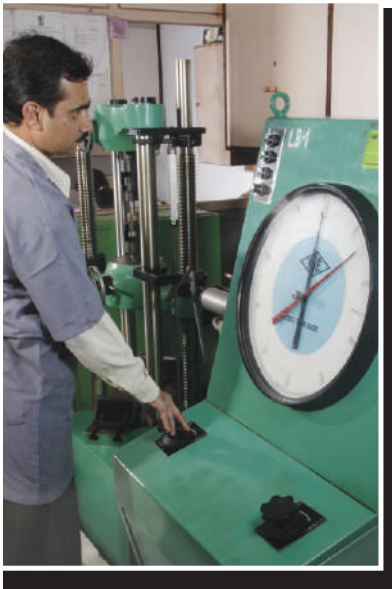
◀ Physical property testing of screws on universal testing machine
