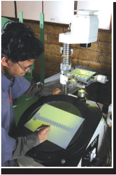
◀ Profile Projector Test for self tapping fasteners
